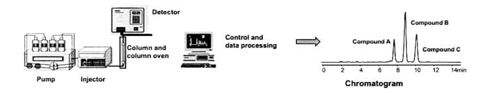
High performance liquid chromatography (HPLC) is a widely accepted separation technique for both sample analysis and purification. It can be utilized in a variety of areas including the pharmaceutical, biotechnological, environmental, polymers and food analysis. (Patania V., 2002).
